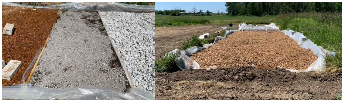
Figure 7b. Media sections of the HTS (L) and the HTS full view (R).
