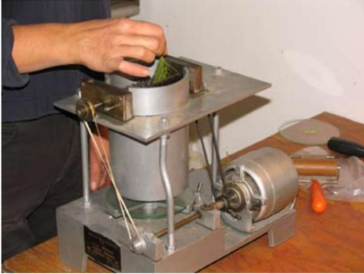
**Figure 4.3** - This piece of equipment is used in counting spider mites. Fine brushes remove mites from foliage where they fall onto a plate. Individuals on the plate are counted. The brushes are thorough, so the counts are very accurate as long as the foliage is collected in such a way that reduces undersampling and sampling bias.
